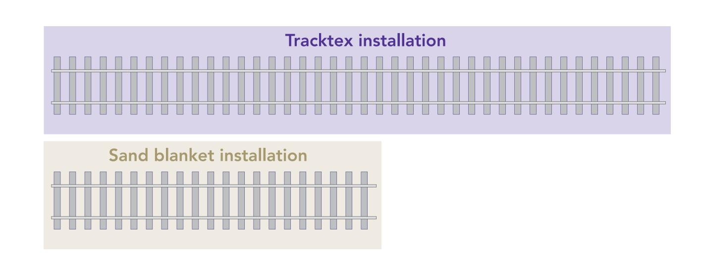
48% more linear metres of Tracktex composite will be installed during a 30hr possession compared with a 100mm thick sand blanket
